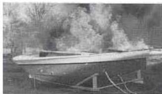
2.5 minutes after ignition of both fire pans. Flame height is over 10 feet, flame temperature is 2150°F
