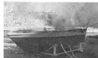
Boat hull after fire test. No structural damage was observed. The hull was insulated by the Flamarest 1600 and kept below its
