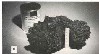
D. Flamarest 1600BTX is a two component catalyzed epoxy intumescent coating. When exposed to heat or flame, the coating intumesces, or swells, to many times its original dry mil thickness. The char that is formed is a low density (less than ½ pound per cubic foot) highly efficient thermal insulator.
